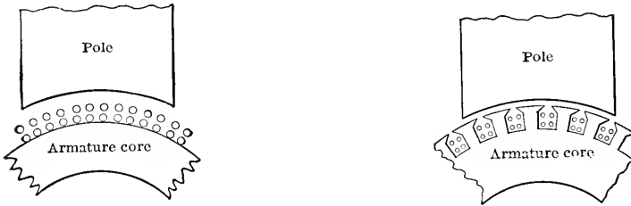
FIG. 149.—The early machines had smooth cores, the winding being placed on the periphery and held in place by binding wires; modern machines always use slotted cores, the windings being imbedded in the slots.
